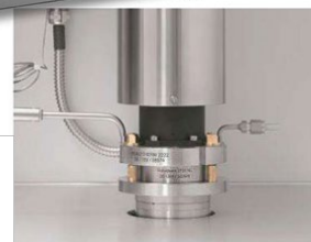
Measuring position: Sealing flange locks for data measurement.
