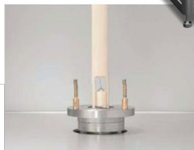
Dispensing position: The sealing flange is open, and the balance head is raised for dispensing.
