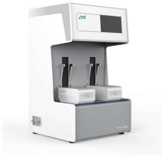
The **Prep 8F** is a versatile, high-throughput degassing system featuring two independent working units, each with four degassing ports, allowing the simultaneous preparation of up to eight samples. Each unit offers independent control of degassing temperature and time, providing flexibility for handling different sample types.
