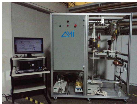
Figure 4. BenchCAT reactor for supercritical trans-esterification of lipids.
