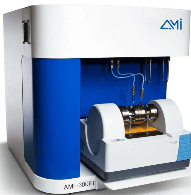
Figure 1. AMI-300 IR shown with integrated Thermo Nicolet iS5 FTIR spectrometer
