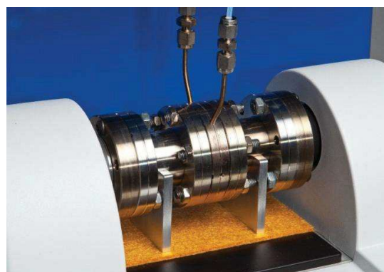
Figure 3. IR transmission cell. Heaters and Insulation have been removed for clarity
