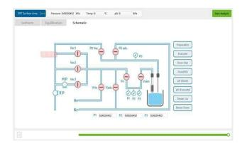
Changes in pressure and temperature inside the manifold can be directly observed in the test interface, providing convenience for sample testing and instrument maintenance. The current state of analyzer can be intuitively understood with the indicator light and event bar.
