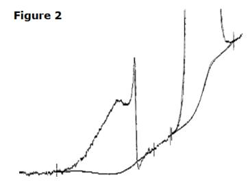
A sample comprised entirely of the higher-melting form shows a single melting peak, without intermediate transitions.
