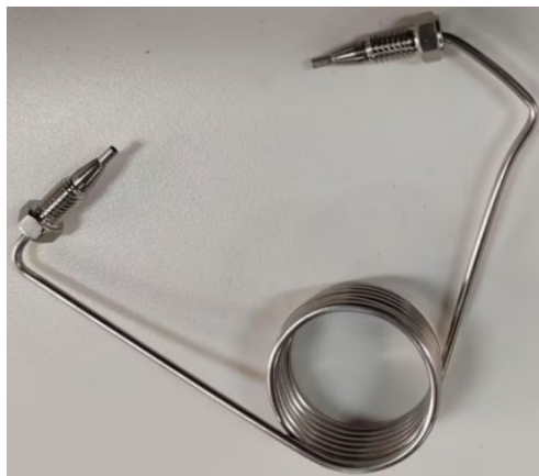
Figure 7. Pulse loops available for the AMI-300 chemisorption system.
